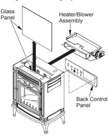
Figure 10 - Removing Glass Panel
